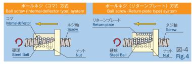
The ball screw consists of a screw spindle, a nut, and steel ball between them (Fig. 4). When the screw is rotated, the ball rolls and moves between the ball screw and the nut, and then returns to its original position. Since a ball is rolled, the friction is low, a high transmission efficiency is obtained, the difference between static friction and dynamic friction is small, and stick-slip does not easily occur.
