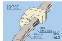
through the circulating hole in the LM block main body, and returns to the other end. Since the sliding surface is fabricated by quenching and abrasive finishing, the rail surface is precise, flat and hard. The ball is set in the pseudo-cylinder shaped groove formed by the sliding surface. Since the pseudo-cylinder surface and the bearing are in contact with each other at two points or four points, slipping does not easily occur.
